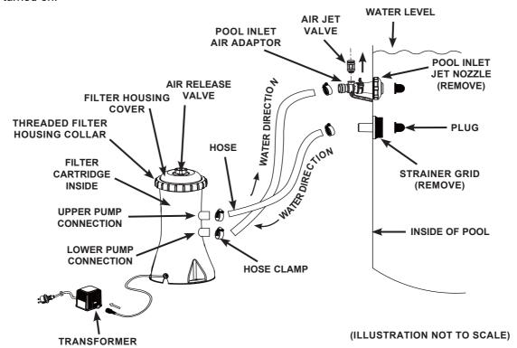
The power cord plug to the 220-240 volt electrical power source of the filter pump must be positioned more than 3.5m away from the pool walls. Check your local authorities to determine the appropriate standard and requirements for "electrical installation of swimming pools and basins equipment". The following table is for reference only:
